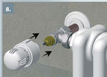
8. Locate the head as shown in the picture by aligning the grooves
